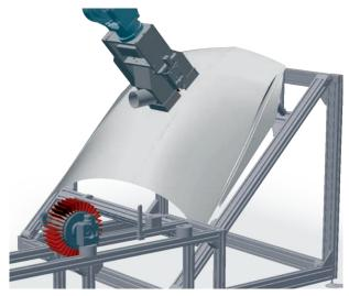
Depending on the product size and application the automated robot can be configured carry the sanding tool and move it relative the stationary processing item, typically larger than 1 meter in any direction
