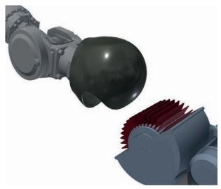
Depending on the product size and application the automated robot can be configured to carry the processing item and move it relative to one or more stationary sanding tools, typically smaller than 1 meter in any direction
